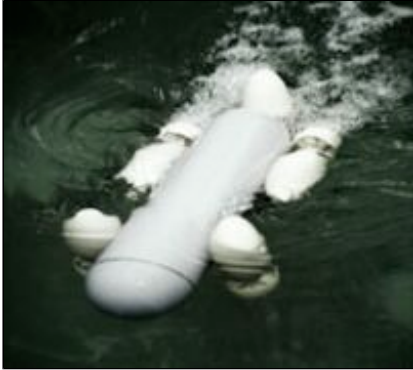
Serafina, the world's smallest autonomous submersible, shows off during a test run.
